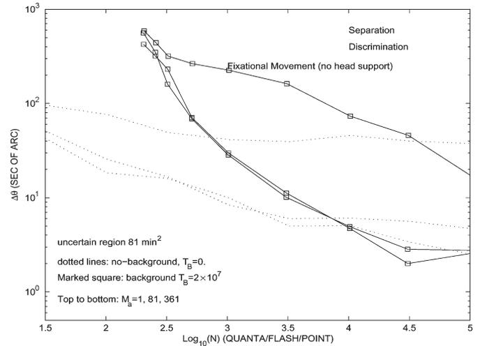
Fig. 9. Threshold for different numbers of SDE observers in the SDS detector, with fixational movement without head support.
