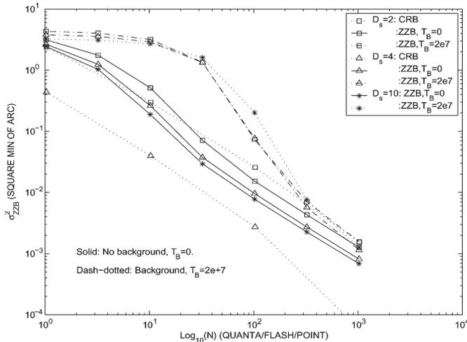
Fig. 15. ZZB for movement estimation accuracy for  $D_s = 2, 4, 10$ , respectively.
