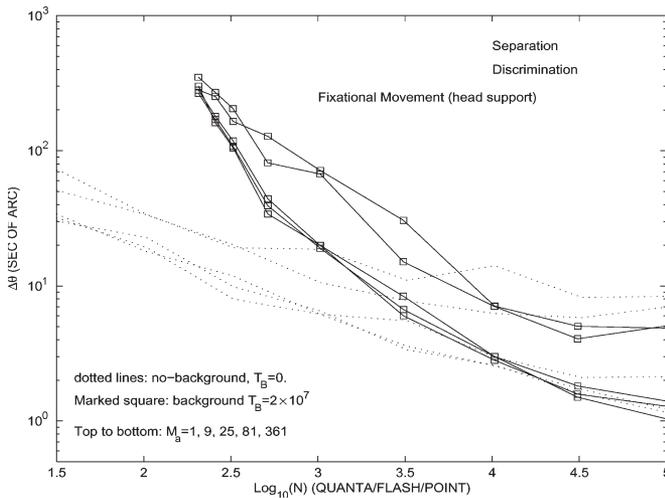
Fig. 8. Threshold for different numbers of SDE observers in the SDS detector, with fixational movement with head support.
